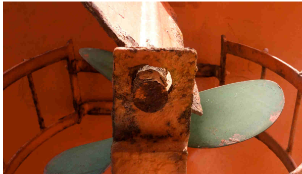
picture 49: worn out rudder shaft of life boat
